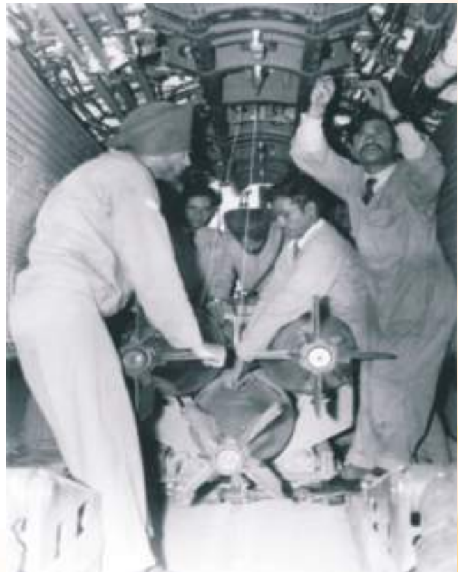
1000lb bombs being loaded in the bomb bay of a Canberra bomber
